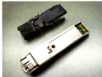
Figure 3. SFF (top) versus optical emSFP (bottom)
